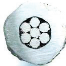
Figure 10 - The Inner Sleeve with 7 Invar Core Strands at the 2nd Cut [1]
