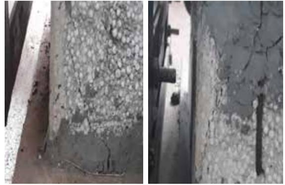
**Figure 7 - Failure Crack Propagation at Core Section in Type 1 Specimens**
