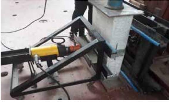
**Figure 4 - Panel Testing of Specimen Type 1 with Connectors**
