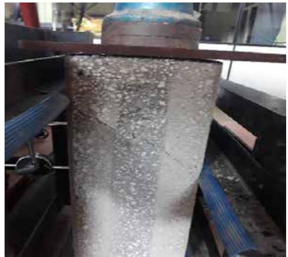
**Figure 8 - Crack Propagation in Type 3 Specimens**
