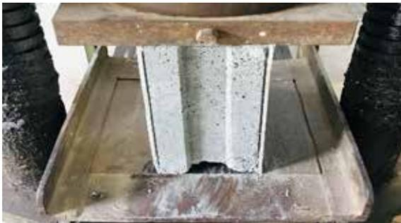
**Figure 17 - Compressive Strength Testing of Panel Specimens**
