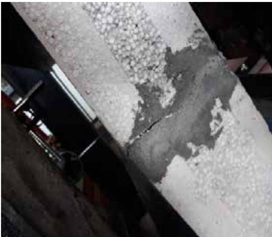
**Figure 6 - First Crack Formation at the Joint in Type 1 Specimens**
