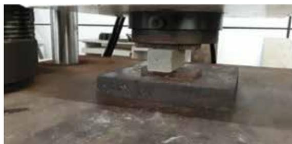
**Figure 1 - Testing for the Compressive Strength**
