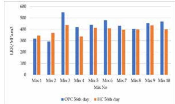
**Figure 18 - Variations of Cost Per Unit Strength for Both Types of Cement (56<sup>th</sup> day)**
