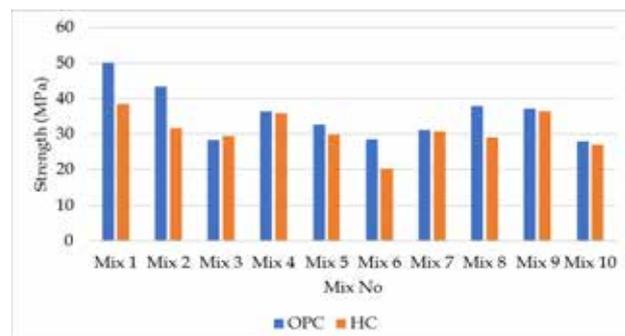
**Figure 10 - Variations of 7-Day Compressive Strength of Cylinders**
