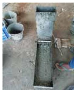
Figure 4 - L-Box test
