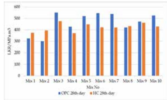
**Figure 17 - Variations of Cost Per Unit Strength for Both Types of Cement (28<sup>th</sup> day)**
