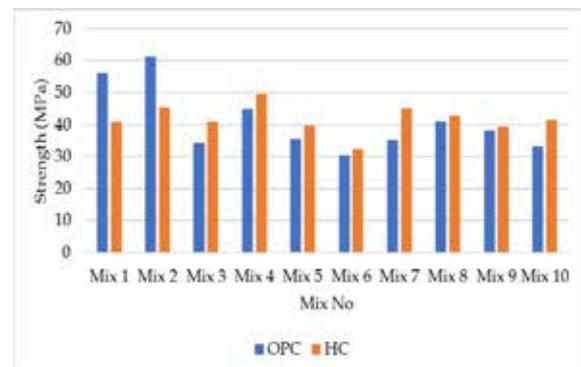
**Figure 12 - Variations of 28-day Compressive Strength of Cylinders**
