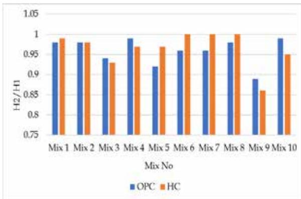
**Figure 8 - Variations of Blocking Ratio of L-Box**
