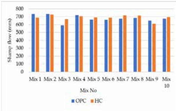
Figure 5 - Variations of Slump Flow
