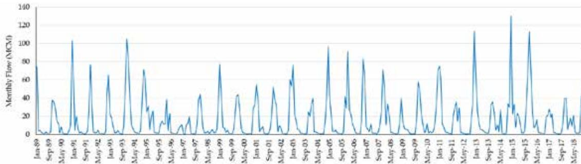
**Figure 11 - Simulated Monthly Flow at Kalu Ganga Dam Site (1989-2018)**
