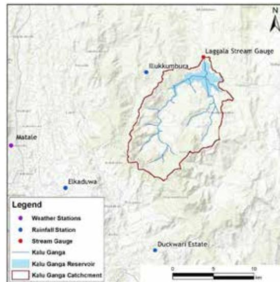
**Figure 4 - Location Details of Meteorological and Stream Gauge Network**
