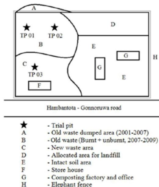
Figure 1 - Layout of the Existing Dump Site
