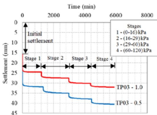
Figure 7 - Settlement-time Curve of New Waste (TP03)
