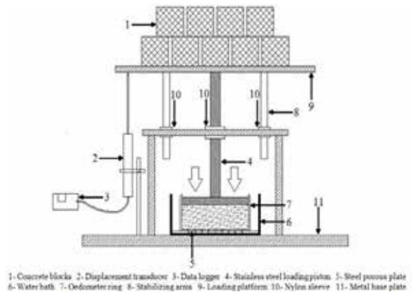
Figure 3 - Cross Section of Experimental Setup
