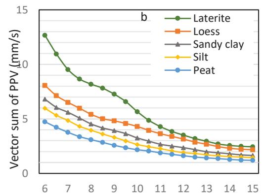
**Figure 6 - PPV of the Ground Vibration With Distance From the Source for Different Soil Types (a) Logarithmic Scale Presentation From 0-15 m Distance (b) Linear Scale Presentation From 6-15 m Distance**
