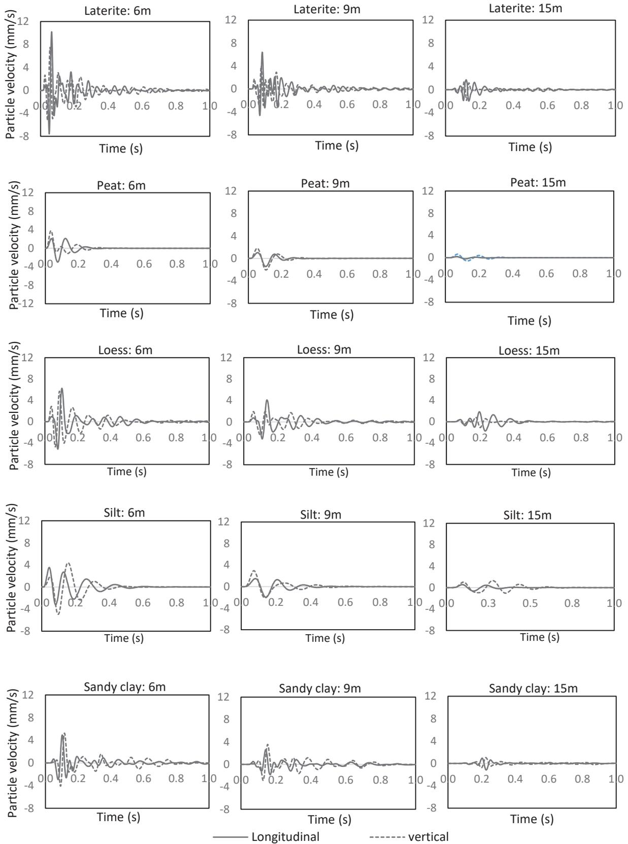
Figure 5 - Wave Propagation at Distance 6m, 9m and 15m in Five Different Soil Types: Laterite, Peat, Loess, Silt and Sandy clay
