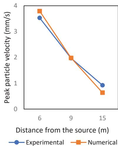
**Figure 3(a) - Experimental and Numerical PPV of Ground Vibration for Peat Soil Measured in the Vertical Direction**
