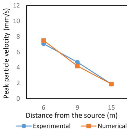
**Figure 4(a) - Experimental and Numerical PPV of Ground Vibration for Laterite Soil Measured in the Vertical Direction**
