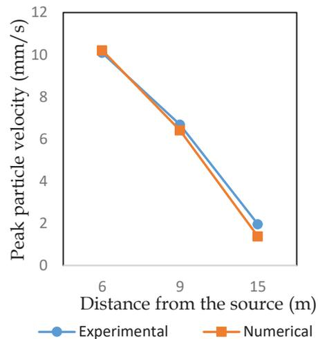
**Figure 4(b) - Experimental and Numerical PPV of Ground Vibration for Laterite Soil Measured in the Longitudinal Direction**
