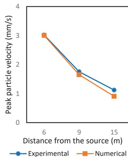
**Figure 3(b) - Experimental and Numerical PPV of Ground Vibration for Peat Soil Measured in the Longitudinal Direction**
