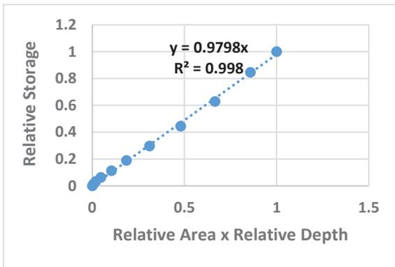
**Figure 5 - Graph of Relative Storage against Relative Area x Relative Depth
