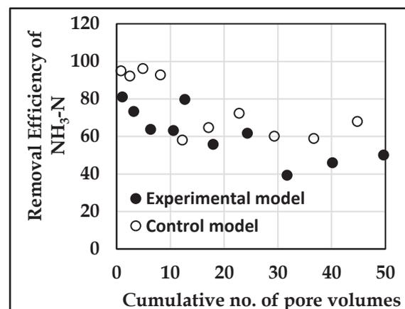
Figure 7 - Variation of NH<sub>3</sub>-N Removal Efficiency
