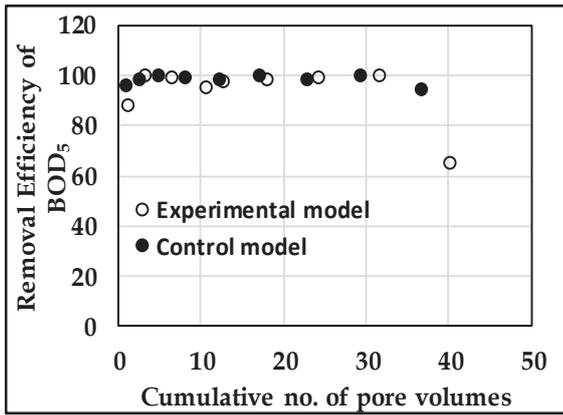
Figure 5 - Variation of BOD<sub>5</sub> Removal Efficiency
