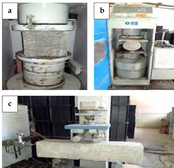
**Figure 1- Testing of Specimens; (a) Compressive Strength Test, (b) Split Tensile Strength Test, (c) Flexural Strength Test**
