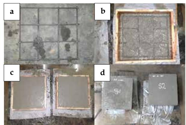
**Figure 2 - Preparation of Slab Panel; (a) Reinforcement Arrangement, (b) and (c) Pouring of Concrete, (d) Curing of Slab Panel**
