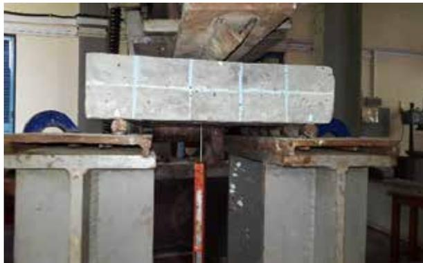
**Figure 4 - Loading Arrangement for the Slab Panel**
