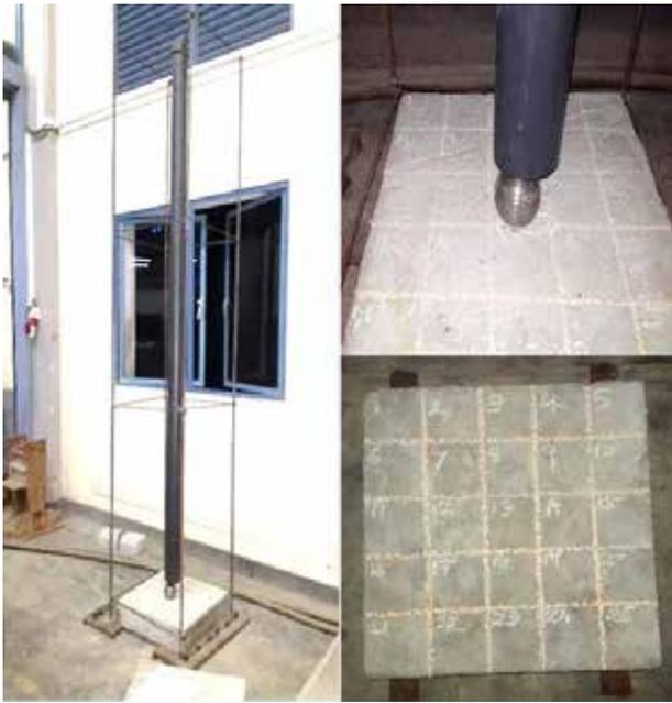
**Figure 3 - Instrumental Set-up for the Impact Resistance Test**
