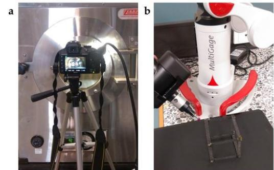
**Figure 5 - Experimental Setup for the Shape Recovery of Deplorable Structure (a) Shape Recovery Process in Vacuum (b) Measuring of Enclosed Volume**
