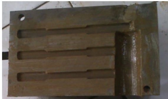
Figure 4 - Cast iron mould designed to prepare specimens for the tensile test and hardness test
