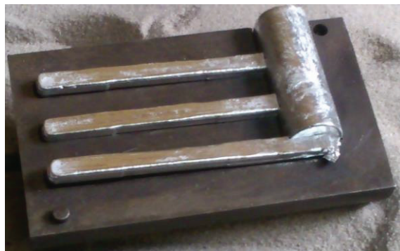
Figure 5 - Al 6063 casting comprising the specimens used in the tensile test and hardness test
