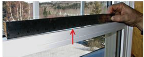
Figure 1 - Deformation in a Al 6063 door frame
