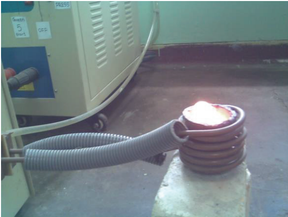
Figure 2 - Melting of Al 6063 Alloy using the induction furnace (IGBT 40)
