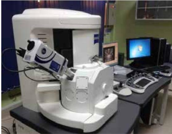
Figure 2- SEM Testing Machine used for the observation
