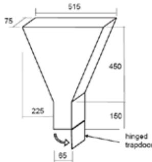
Figure 4(b) - V-Funnel test: Time taken to empty the funnel is taken as measure of flow ability (Segregation resistance) of the mix
