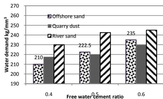
Figure 10 - Water demand by different aggregate types at different w/c ratio at 70% fine aggregate proportion
