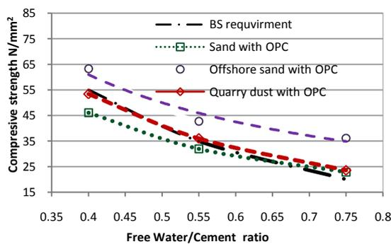
Figure 14 - Average strength vs. water cement ratio for Normal Concrete
