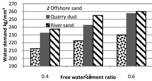
Figure 11- Water demand for different aggregate types with common particle size distribution operated at 70% of fine aggregate proportion
