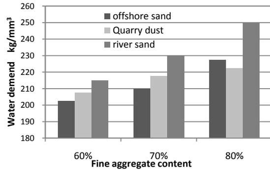
Figure 8 - Increase in water demand with the increase in aggregate proportions recorded for W/C ratio of 0.4.
