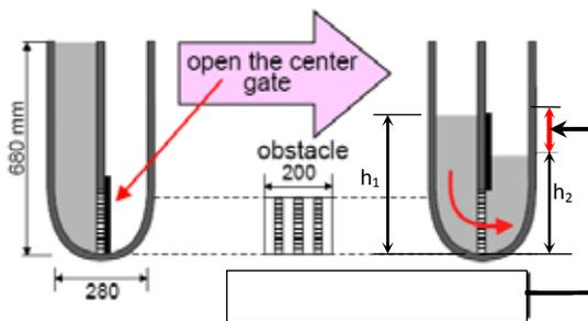
Figure 4(a) - U box test: Difference in the two legs is taken as a measure of the flow ability (passing ability) of the concrete mix
