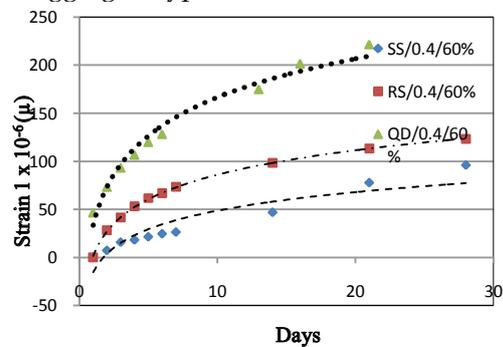
Figure 16- Typical shrinkage measurement of SCC for various aggregate types
