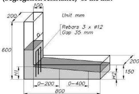
Figure 4(c) - L box test: Ratio or difference in the height of the horizontal leg of the mould measure the passing ability of SCC.
