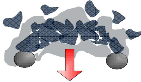
**Figure 2(b) - Aggregate arch blocking the passing ability in SCC**
