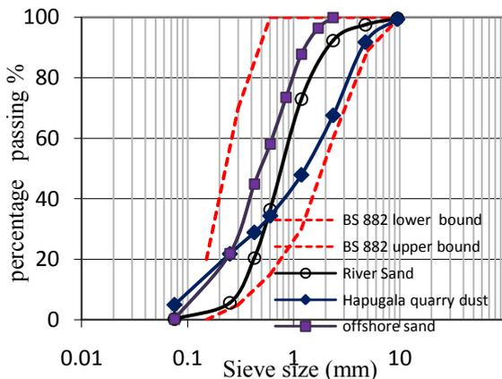
Figure 6 - Particle size distribution of different fine aggregate types compared with the upper and lower bounds of the BS882 requirement for concrete.
