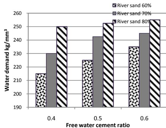
Figure 9 - water demand with the increasing water/cement ratio
