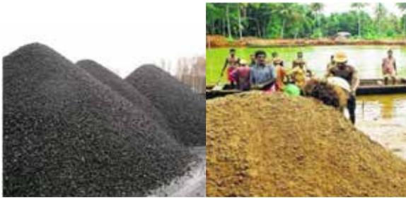
Usual coarse aggregate (Crushed stones) and fine aggregate (River sand) for concrete
