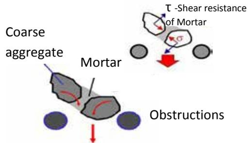
**Figure 2(a) - Forces acting on the coarse aggregate**
