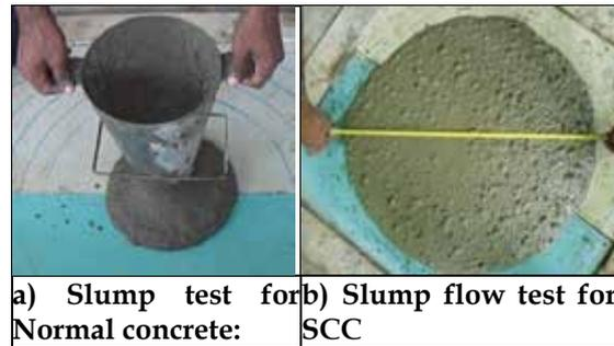
**a) Slump test for Normal concrete:      b) Slump flow test for SCC**
