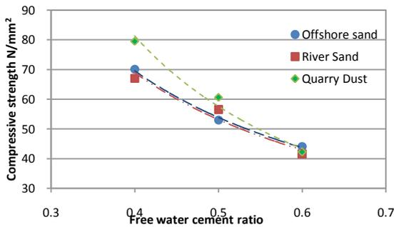
Figure 13 - Average strength vs. water cement ratio for SCC
