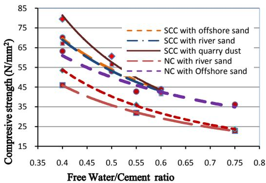
Figure 15 - Strength vs. w/c ratio for the three aggregate types for normal and self-compacting concrete.
