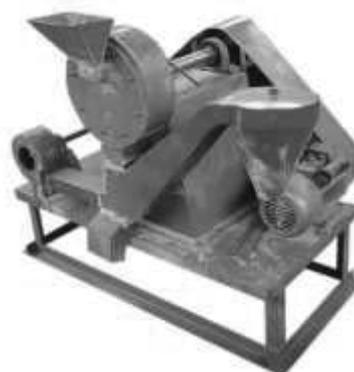
Photograph 2- Fabricated Rasp bar mill
