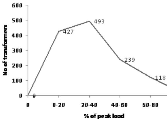
**Figure 6.2 - Number of transformers with percentage peak loading**
