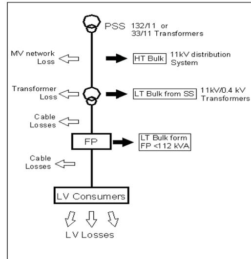
**Figure 6.1 - Schematic diagram of electricity distribution system of Colombo City**
