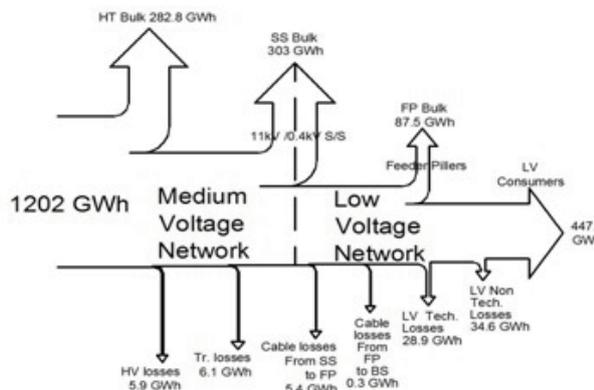
**Figure 6.4 -Energy flow diagram of Colombo City for the year 2009**
