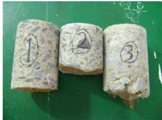
Figure 1- Concrete core samples
