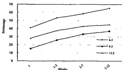
Figure 3 Cumulative Percent of aggregates loss after initial count
