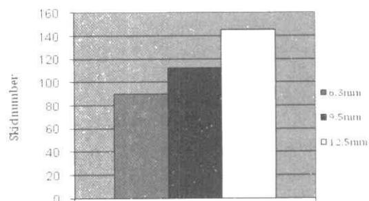
**Figure 5 Skid numbers of three chip sizes**
