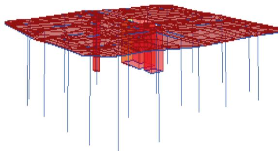
Figure 01: Column layout below the transfer plate
