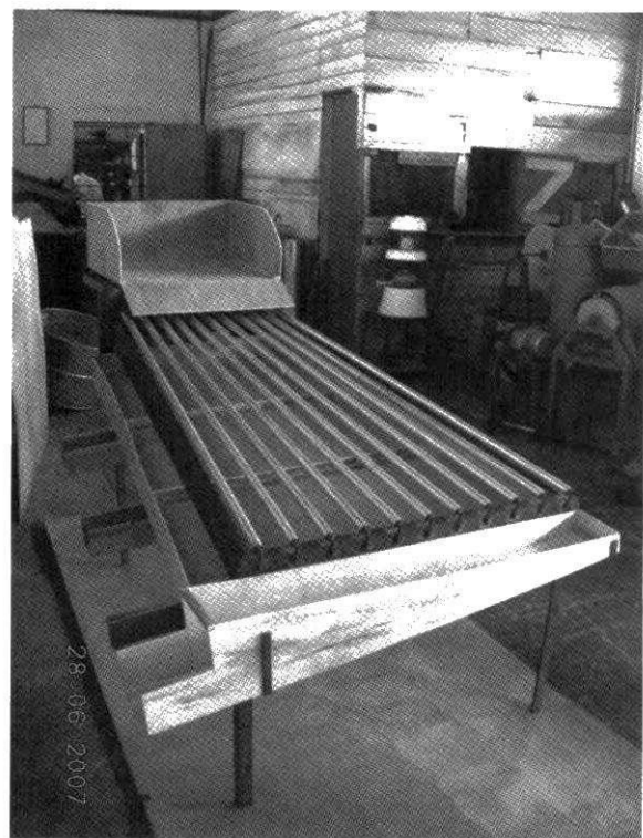
Figure 3: Fabricated chutes and hopper with plywood
