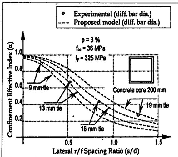
Figure 6. Model prediction of experimentally evaluated confinement effectiveness index for different tie stiffnesses
