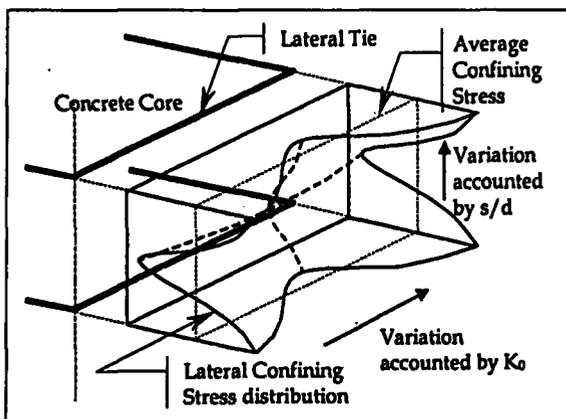
Figure 1. Confining stress distribution by discretely spaced ties
