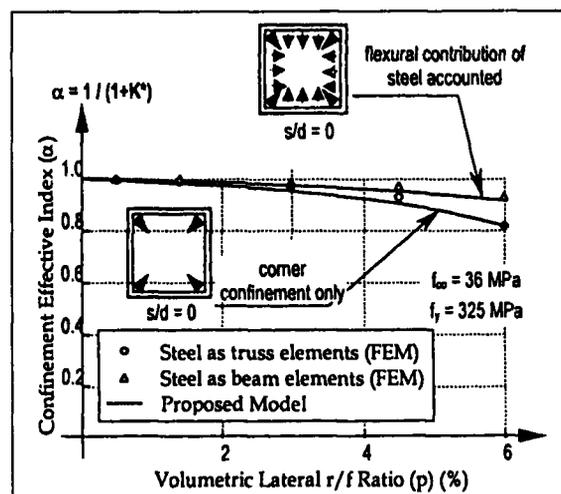
Figure 4. Limit uniformity factor (detailing)
